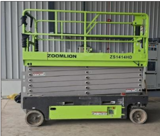
SCISSORS LIFT ZS1414HD (MAX HEIGHT 15,7M)
