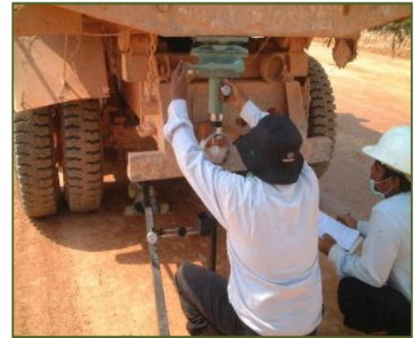
CBR Test on Site
