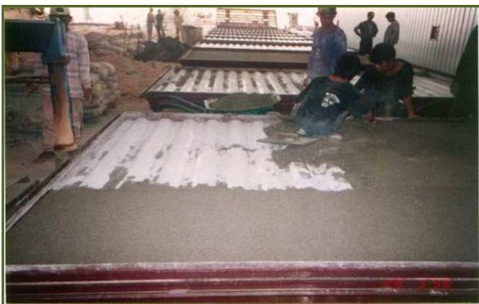
Vermiculite Heat Insulation for Kiln Cars
