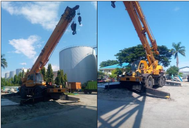
Mobile Crane QY25K XCMG 25 ton
