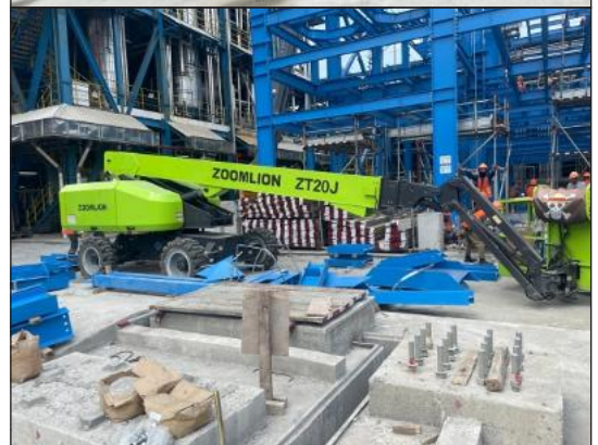
Boomlift Zoomlion ZT20J Capacity : 300kg
