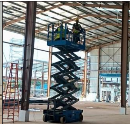
SCISSORS LIFT GS-3246 (MAX HEIGHT 11,78M)
