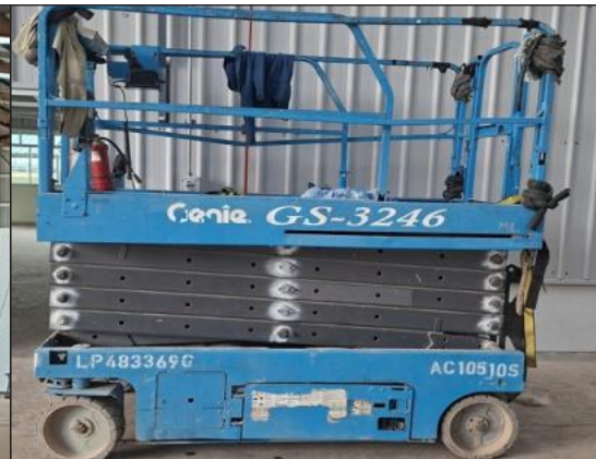
SCISSORS LIFT GS-3246 (MAX HEIGHT 11,78M)
