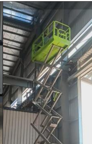
SCISSORS LIFT ZS1414HD (MAX HEIGHT 15,7M)
