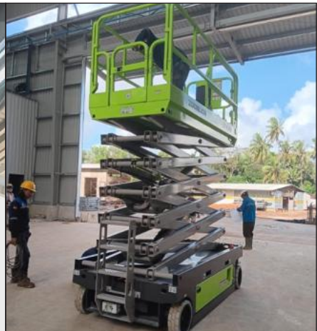
SCISSORS LIFT ZS1414HD (MAX HEIGHT 15,7M)
