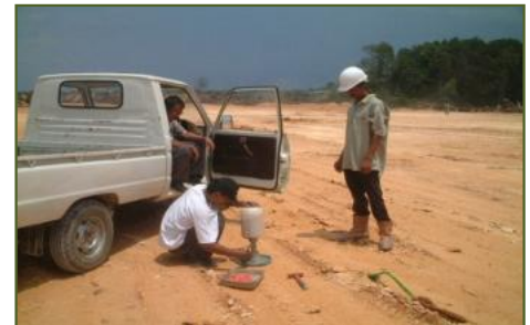
Sand Cone Test
